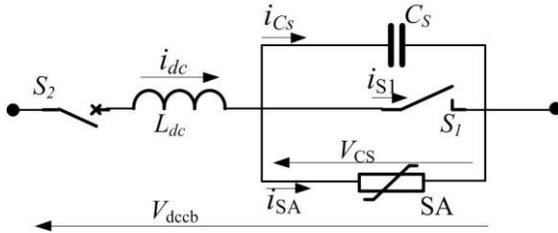
Figure 1. Topology of series LC DC Circuit Breaker.
