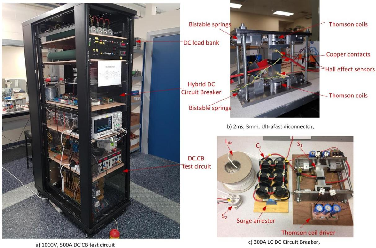
Figure 3. Laboratory demonstrator: a) 900V DC CB test circuit, b) 3 mm, 2 ms fast air disconnector, c) Series LC DC Circuit Breaker.
