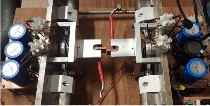
Figure 4. Internal view of contacts assembly of fast disconnecter.
