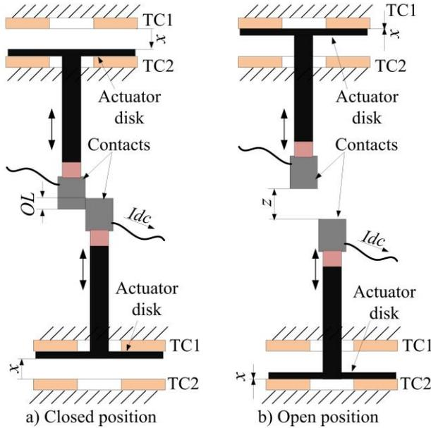
Figure 2. Fast disconnector with lateral contact overlap.
