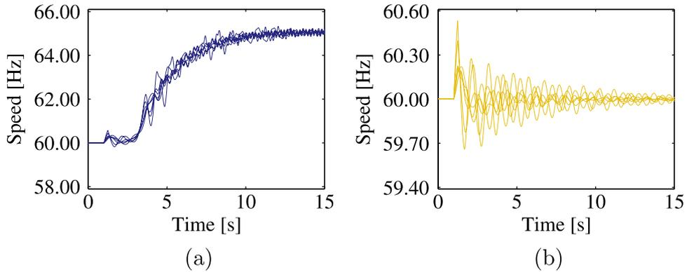
**Figure 3.** Turbine speeds during a bus fault at bus 12 that starts at the 1 second mark and lasts for 0.23 s ( $t_{ccl} = 0.2276$  s without ACVGs). The line colors correspond to deviation from the nominal value of 60 Hz. Parameters that deviate strongly are colored purple (dark gray), while those with minor deviations are colored yellow (light gray). Without ACVGs the system fails to resume synchronous operation (a) as opposed to the situation when ACVGs are used (b).
