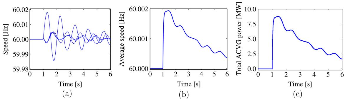
**Figure 1.** Changes in the turbine speeds due to a sudden load decrease of 10% at bus 20 which starts at the 1 s mark (a). As expected, the lack of load leads to a surplus in power which results in increased average speed (b). This change is quickly met by the ACVGs which act as loads in order to absorb the excess power (c).
