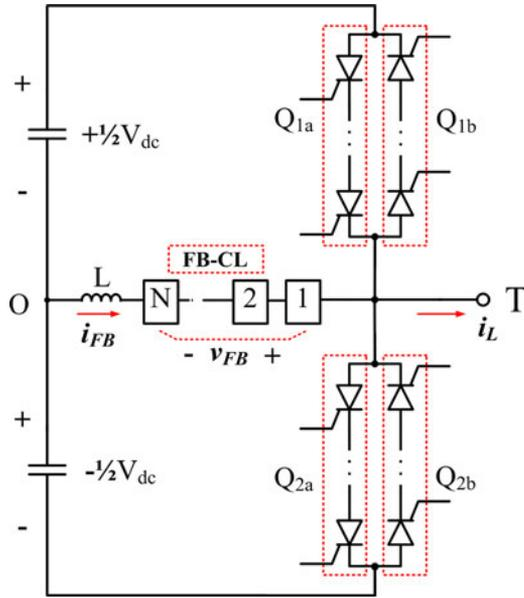
Fig. 1. Proposed AFC-bridge using hybrid power devices.
