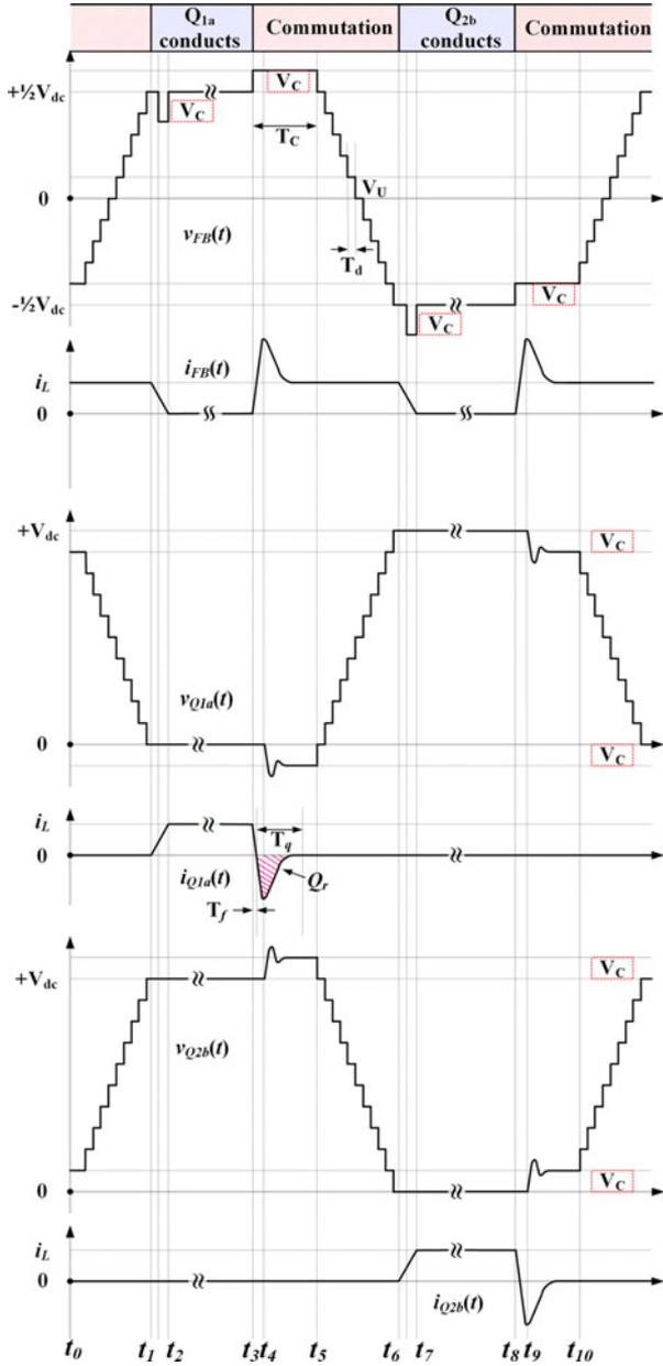
Fig. 2. Commutation of the AFC-bridge (when load current  $i_L > 0$ ) with FB-CL operating in CPST mode.
