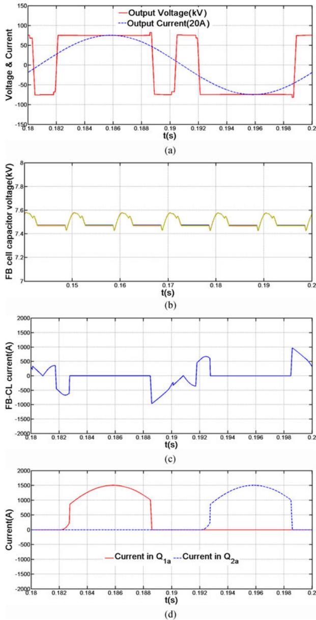
Fig. 6. Key waveforms of the AFC-bridge: (a) output voltage and current; (b) FB capacitor voltage balancing; (c) FB-CL current; and (d) current carried by thyristor  $Q_{1a}$  and  $Q_{2a}$ .
