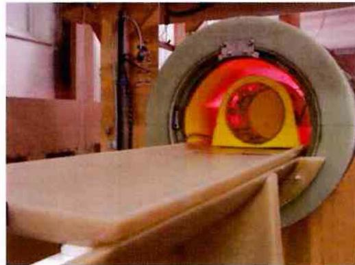
**Figure 1:** View of the whole-body 0.2 T FFC-MRI scanner with a home-made head coil inside the bore.
