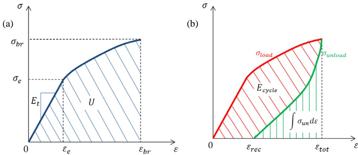
201 **Fig. 3** Representation of stress-strain curves for: tensile test at breakage (a) and tensile cyclic loading-unloading test (b). The
