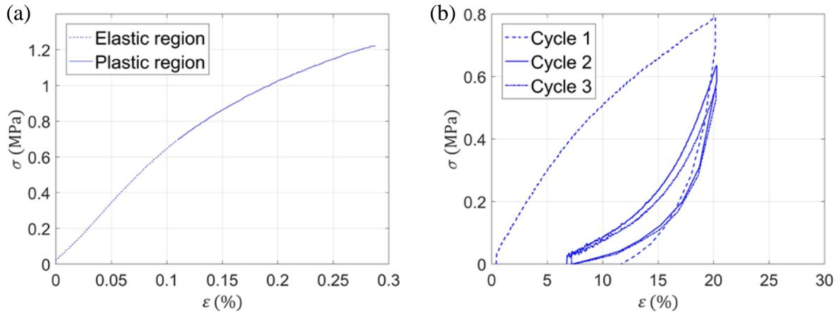
365 **Fig. 6** Examples of stress-strain curves from a tensile test up to the breakage point (a) and a tensile cyclic loading-unloading
