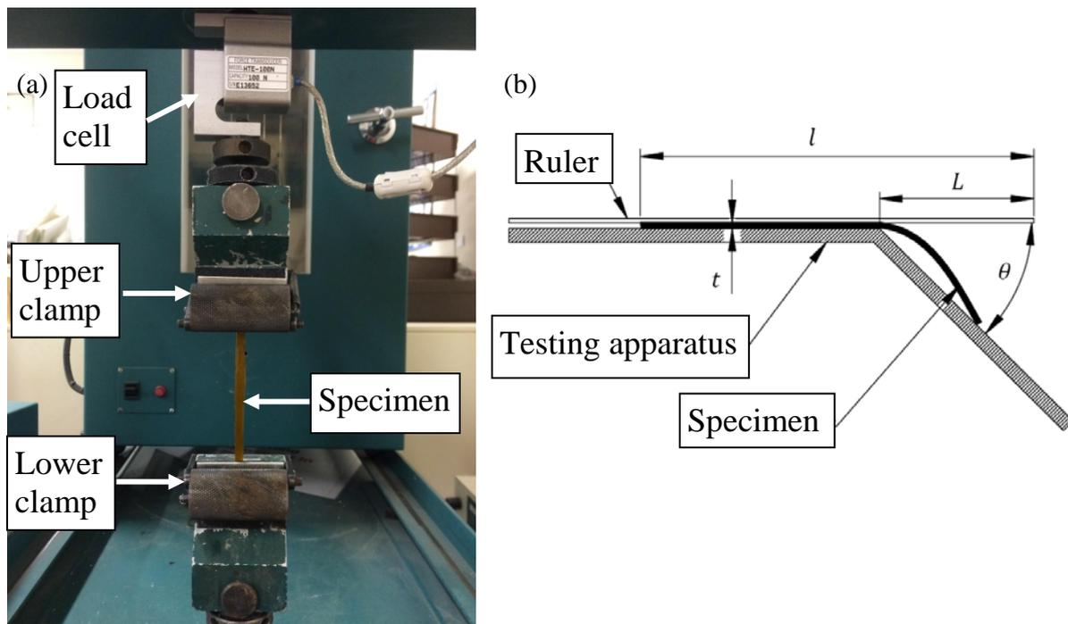
172 **Fig. 2** Hounsfield S-series benchtop testing machine during the testing of a seaweed blade specimen (a). Schematic
