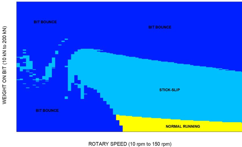
**Figure 2.** Stability map of stable (normal running) and unstable responses (stick-slip and bit bounce) computed for the fully nonlinear system. The system parameters were chosen the same as given in Table 1 of [4].
