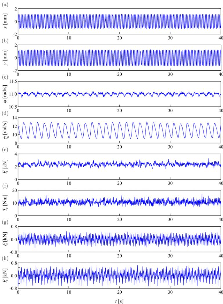
**Figure 3.** A sample of the recorded experimental time histories for configuration with 20 disks; (a) and (b) displacement of the BHA in the  $x$  and  $y$  direction respectively, (c) and (d) top and bottom speed, (e)  $F_z$ , (f)  $T_z$ , (g) and (h) transverse forces on  $x$  and  $y$  direction acting on the drill-bit.
