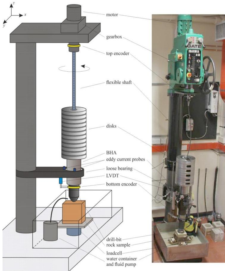
**Figure 3.** A schematic (left) and photograph (right) of the Aberdeen Drill-String Dynamics Experimental Rig showing its main components such as BHA, flexible shaft, WOB disks, drill-bit, rock sample and motor. The instrumentation include a 4D load-cell, LVDT, top and bottom encoders and eddy current probes.
