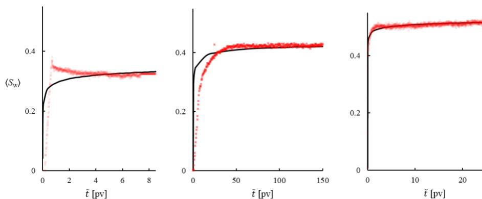
**Fig. 4.** Evolution of the remaining oil saturation as measured in the packed bed (red  $\times$ ) and simulated by history matching (solid line) for  $Ca = 1.5 \times 10^{-6}$  (left, M8),  $4.6 \times 10^{-5}$  (middle), and  $2.2 \times 10^{-4}$  (right). Where the solid line is not visible, it overlaps with the markers.
