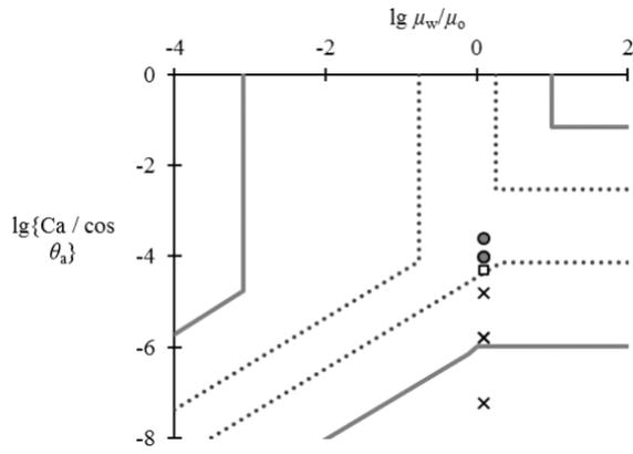
**Fig. 2.** Mobility ratio-Ca regime map. Marker shapes depict flow patterns observed in the displacement experiments: capillary fingering (cross), stable displacement (solid circle), and post-breakthrough sweep (squares). Superposed are regime boundaries for primary drainage proposed in the literature for uniformly wetting micromodels: a network of capillaries ([1], grey solid line) and a uniform cylinder array ([2], grey dotted). Adapted from [16].
