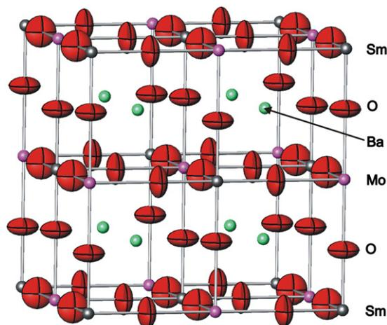
**Fig. 6.** The crystal structure of  $\text{Ba}_2^{154}\text{SmMoO}_6$ ; Sm, Mo, Ba and O atoms are labelled. The ellipsoids on the oxygen sites evidence a transverse thermal motion.
