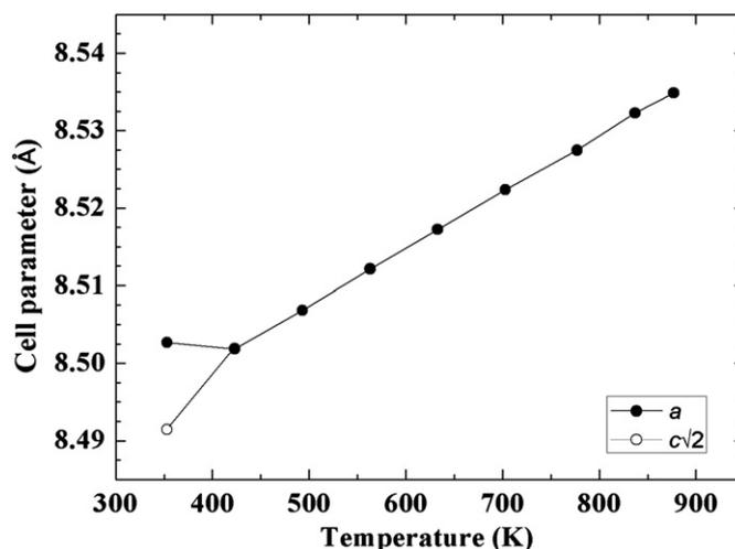
Fig. 4. Evolution of the cell parameters with temperature in  $\text{Ba}_2^{154}\text{SmMoO}_6$  evidencing a structural distortion at 353 K,  $c$  is multiplied by  $\sqrt{2}$  for comparison purposes.
