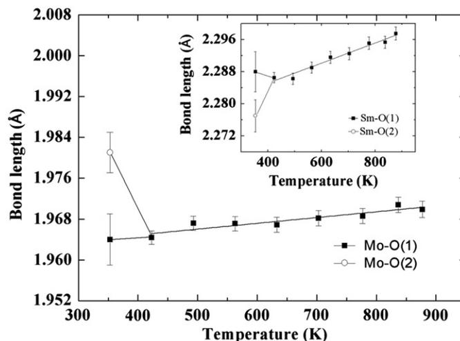
Fig. 3. Evolution of the Mo–O and Sm–O (inset) bond lengths with temperature in  $\text{Ba}_2^{154}\text{SmMoO}_6$ , showing a cubic–tetragonal structural transition at 353 K.
