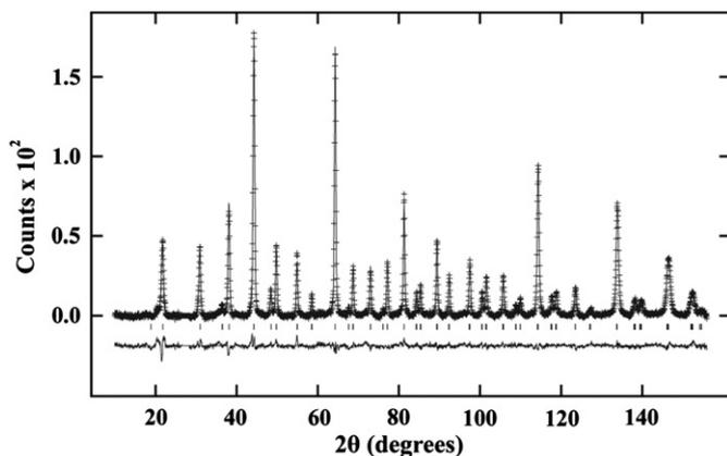
Fig. 1. Rietveld refinement fit to the 353 K neutron diffraction pattern of  $\text{Ba}_2^{154}\text{SmMoO}_6$ . Data is excluded in the  $2\theta$  range  $26.5^\circ$ – $28.35^\circ$  to account for a peak associated with the cryofurnace.
