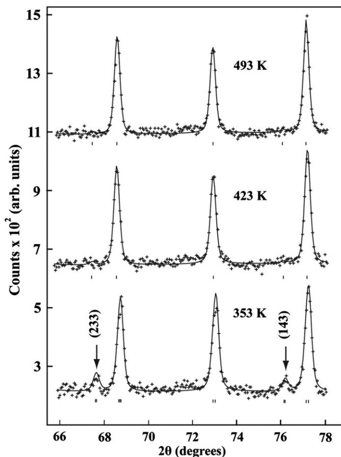
Fig. 2. A portion of the refined neutron diffraction pattern of  $\text{Ba}_2^{154}\text{SmMoO}_6$  between  $66^\circ$  and  $78^\circ$   $2\theta$  evidencing a cubic–tetragonal structural distortion between 423 and 353 K. Data is fit to the tetragonal  $I4/m$  space group at 353 K and cubic  $Fm-3m$  above this temperature.
