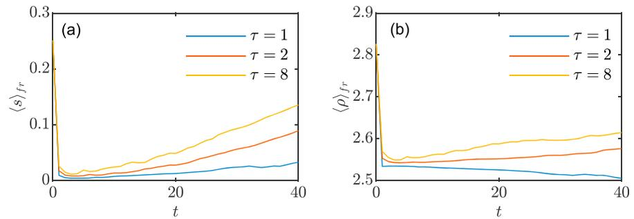
**Figure 4.** Average salinity (a) and density (b) in the frontal region of the current, where the sediment concentration  $c > 0.9$ . The large initial values represent an artifact, as no well-developed front has formed yet. Differential diffusivity is seen to increase the density of the frontal region of the current.
