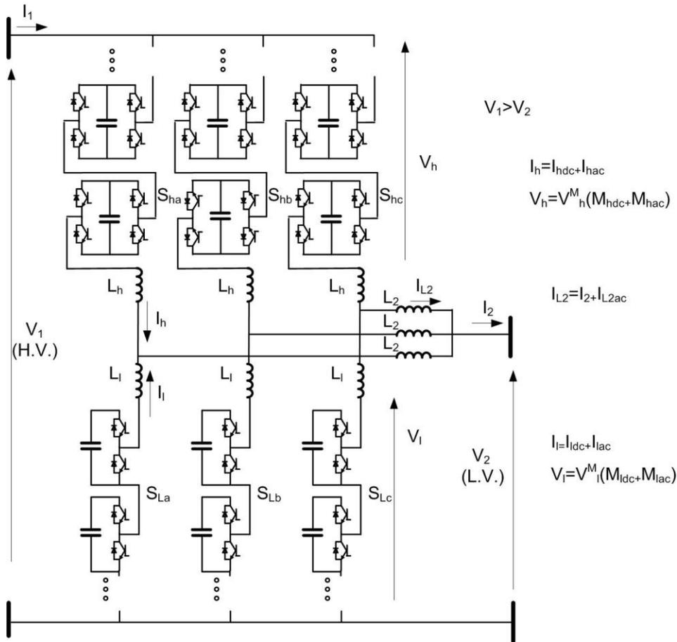
Figure 1. Topology of non-isolated DC/DC converter.
