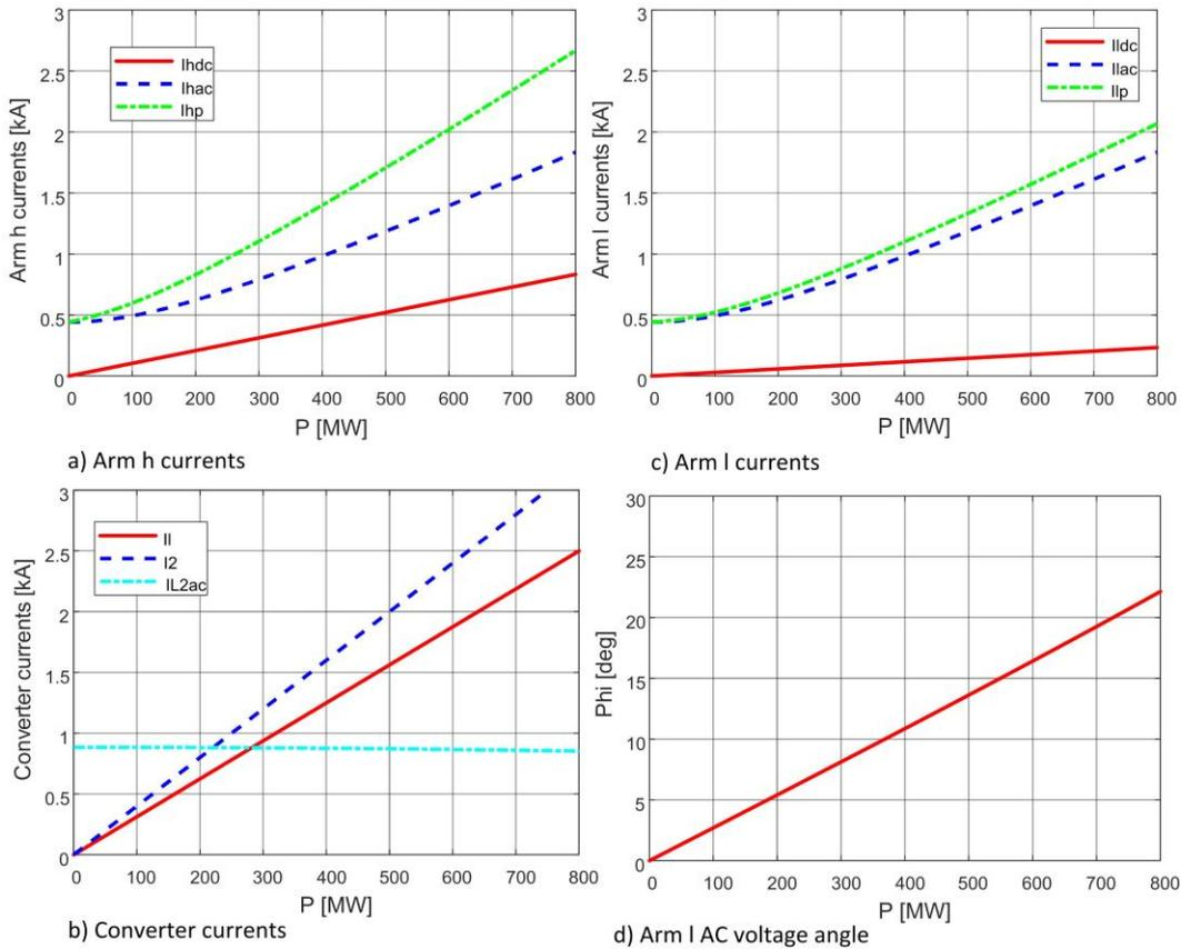
Figure 2. Design variables as power rating is changing ( $V_1=320kV$ ,  $V_2=250kV$ ,  $f=150Hz$ )
