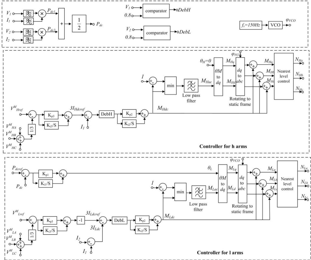
Figure 3. Controller for Non-Isolated MMC DC-DC.
