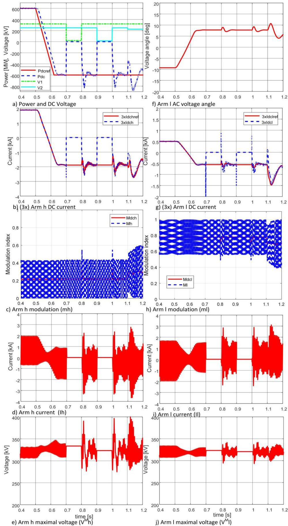
Figure 4. Converter response for power reversal, DC faults and V2 step reduction.
