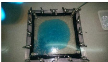
**Figure 7.** Failed trial run, February 2016. The injected aqueous solution (blue) forced its way through a gap between the packed bed and the top of the Hele–Shaw cell because the cell was not packed fully.
