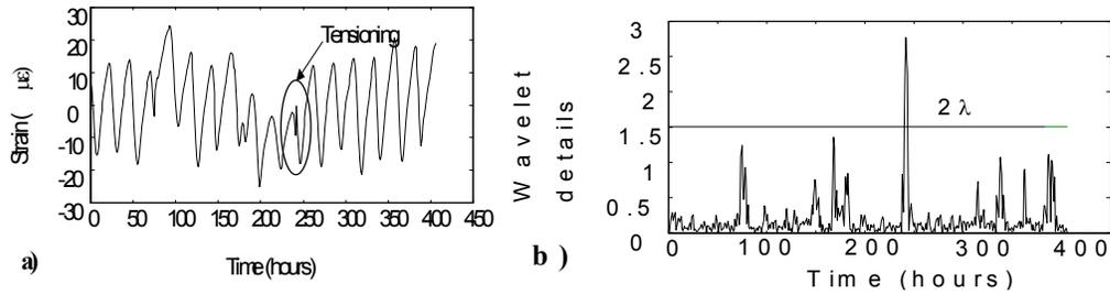
**Figure 3. Tensioning of a bridge segment during construction: a) strain time series, b) wavelet detail coefficients at lowest scale**
