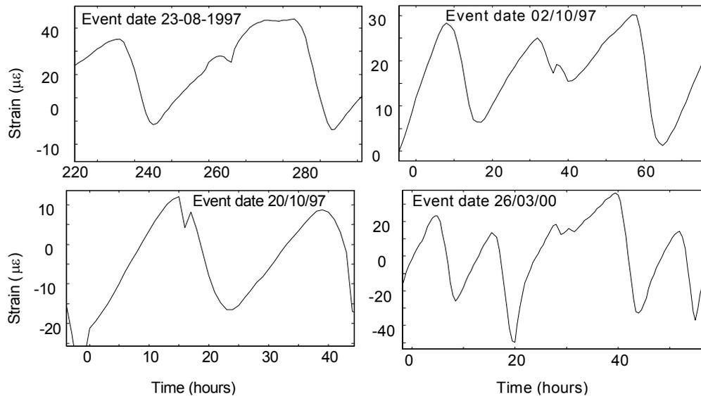
**Figure 4. Abrupt events identified during post-construction stage.**
