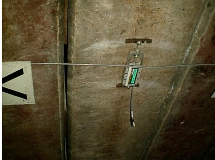
**Figure 3 – Demountable strain gauge attached to bridge soffit.**
