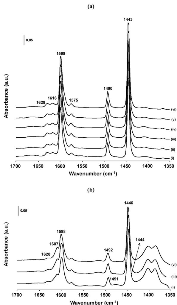
Fig. 4. Difference spectra after and before pyridine adsorption in the 1700–1350  $\text{cm}^{-1}$  FTIR region for the (a) Na-exchanged and (b) magnesium-impregnated zeolites: (i) parent zeolite and desiccated zeolites at (ii) 0.01, (iii) 0.02, (iv) 0.05, (v) 0.1 and (vi) 0.2 M.
