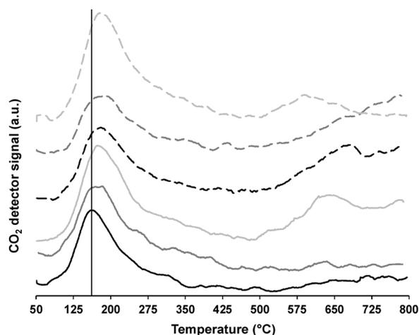
Fig. 8.  $\text{CO}_2$ -TPD results for the magnesium-impregnated zeolites: 5%MgNaY (black line), 5%MgNaY<sub>0.01</sub> (dark grey line), 5%MgNaY<sub>0.02</sub> (light grey line), 5%MgNaY<sub>0.05</sub> (dashed black line), 5%MgNaY<sub>0.1</sub> (dashed dark grey line) and 5%MgNaY<sub>0.2</sub> (dashed light grey line).
