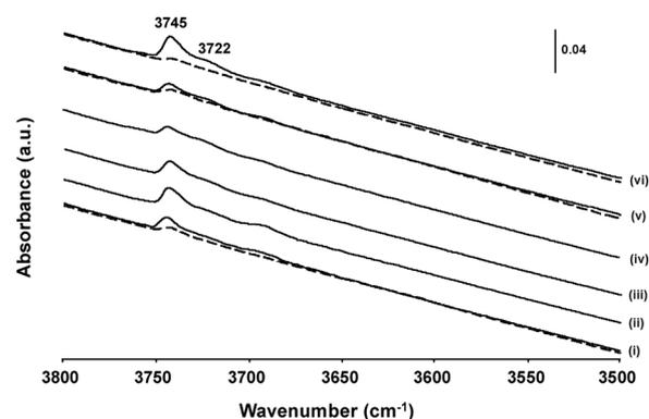
Fig. 3. 3800–3500  $\text{cm}^{-1}$  region of the FTIR spectra for the (i) parent zeolites and desilicated zeolites at (ii) 0.01, (iii) 0.02, (iv) 0.05, (v) 0.1 and (vi) 0.2 M. Na-exchanged samples (black lines) and magnesium-impregnated samples (dashed lines).
