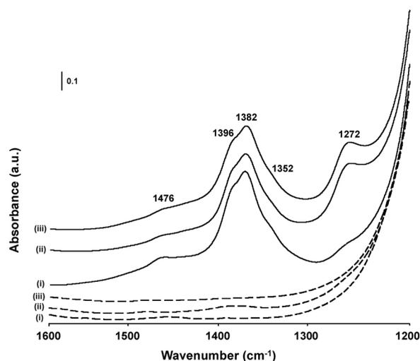
**Fig. 6.** 1600–1200  $\text{cm}^{-1}$  region of the FTIR spectra for the magnesium-impregnated samples (black lines): (i) parent zeolite and desilicated zeolites at (ii) 0.05 and (iii) 0.2 M. Dashed lines – spectra of Na-exchanged zeolites for comparison.
