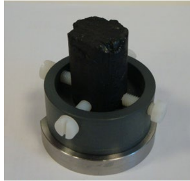
100 101 Figure 1. Coal core sample in a sample holder used in this study.
