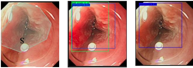
Figure 8. Illustration of removing duplicated boxes labelled with different classes using NMS approach when overlapping exceeding 80%. The example showing the result from YOLOv3.
