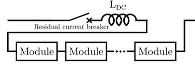
Fig. 7. VARC DCCB circuit diagram. The module block contains the circuit shown in Fig. 6.
