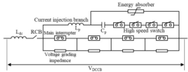
Fig. 4. Detailed active current injection DCCB model
