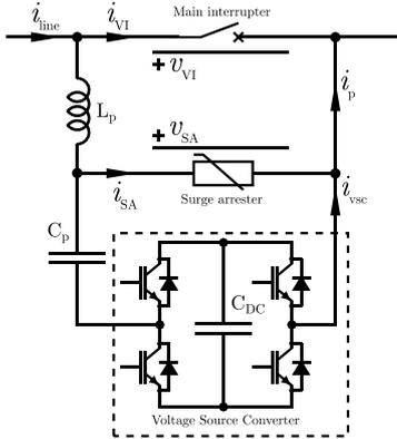
Fig. 6. Main circuit diagram of a VARC DCCB module
