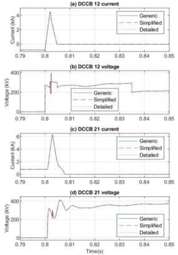
Fig. 9. Voltage and current responses of three HCB models
