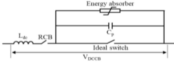
Fig. 5. Simplified active current injection DCCB model
