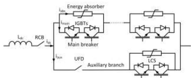
Fig. 1. Detailed equivalent HCB model
