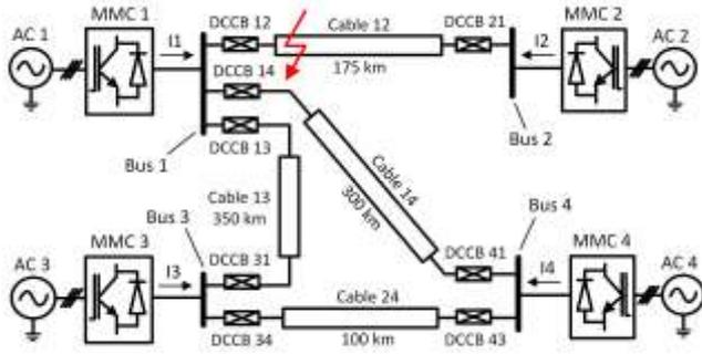
Fig. 8. Four terminal DC grid test system
