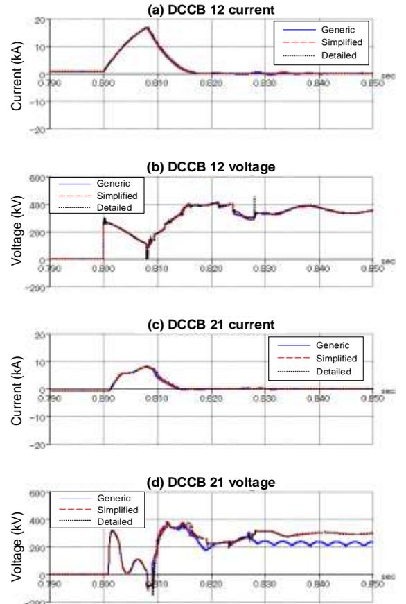
Fig. 10. Voltage and current responses of three active current injection DCCB models
