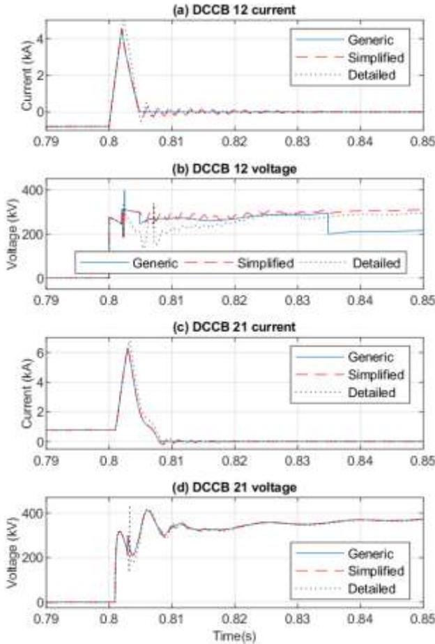
Fig. 11 Voltage and current responses of three VARC DCCB models
