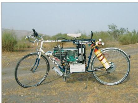
Figure 4 Fuel-cell-powered bicycle
