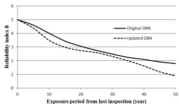
**Fig. 4:** Predicted reliability of pipeline failure for an exposure period of 50 years.
