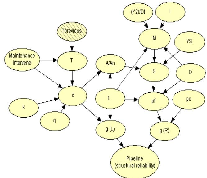
Fig. 3: Structural reliability of pipeline as a DBN.
