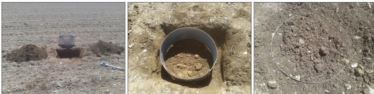
Fig. 2 Root exclusion collars (n = 8) dug into the land-use change areas following the soil disturbance of cultivation and planting.
