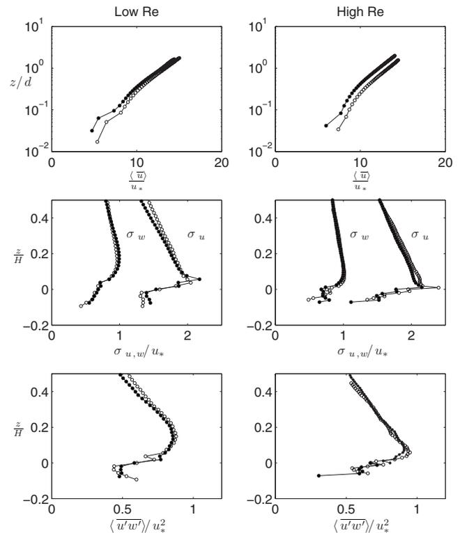
FIG. 4. Spatially averaged flow statistics. Open and filled symbols stand for one and five layer beds, respectively;  $\sigma_u = \sqrt{\langle \bar{u}'^2 \rangle}$ ;  $\sigma_w = \sqrt{\langle \bar{w}'^2 \rangle}$ ;  $H$  is the flow depth;  $u_*$  is the shear velocity as defined in Table I.
