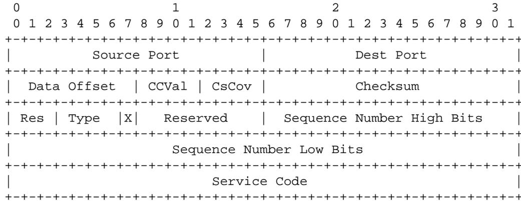
Figure 1: Format of a DCCP-Listen Packet
