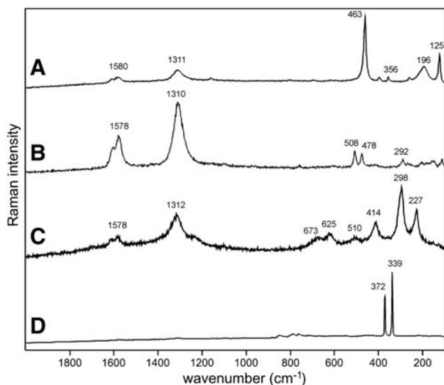
**FIG. 4.** Sample 4 (785 nm excitation). (A) Clear signatures of disordered carbon (1300–1600  $\text{cm}^{-1}$ ) and quartz (below 500  $\text{cm}^{-1}$ ); (B) strong disordered carbon signal with two peaks of feldspar and very weak features of hematite (below 600  $\text{cm}^{-1}$ ); (C) disordered carbon and clear hematite features below 700  $\text{cm}^{-1}$ , note the shoulder at around 1320  $\text{cm}^{-1}$  representative of disordered hematite; (D) pyrite.
