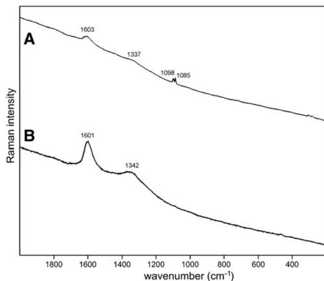
**FIG. 8.** Sample 8 (514.5 nm excitation). The sample was fluorescent at 785 nm, and slope of fluorescence is present also when 514.5 nm excitation was used, but with observable Raman features. (A) Matrix with calcite and dolomite peaks 1086 and 1098  $\text{cm}^{-1}$ , respectively (calcite is prevailing through the sample); very broad features of disordered carbon are present as well between 1300 and 1650  $\text{cm}^{-1}$ . (B) Broad Raman features of disordered carbon.
