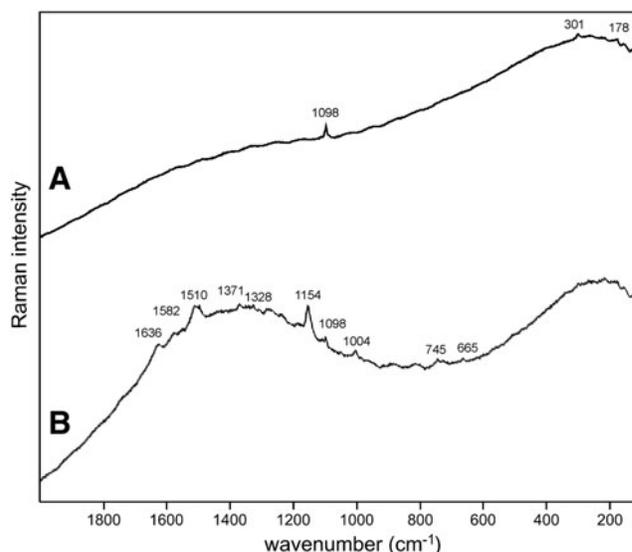
FIG. 3. Sample 3 (785 nm excitation). (A) Dolomite signal with relative high fluorescence background; (B) bands of three different pigments are evident on fluorescence background between  $600\text{ and }1650\text{ cm}^{-1}$ —carotenoid, chlorophyll, and phycobiliproteins, which are typical for cyanobacteria.
