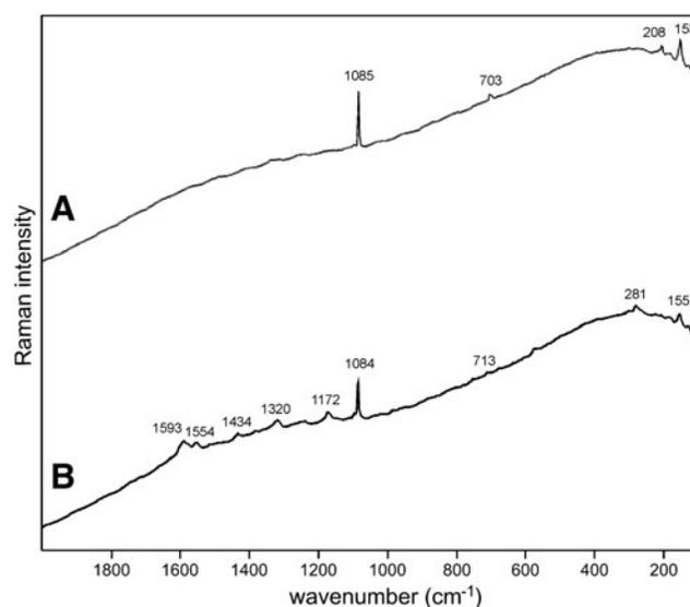
FIG. 2. Sample 2 (785 nm excitation). (A) Aragonite matrix; (B) aragonite with clear features of UV-protective pigment scytonemin between  $1150\text{ and }1600\text{ cm}^{-1}$  corroborated by weak bands below  $800\text{ cm}^{-1}$ .
