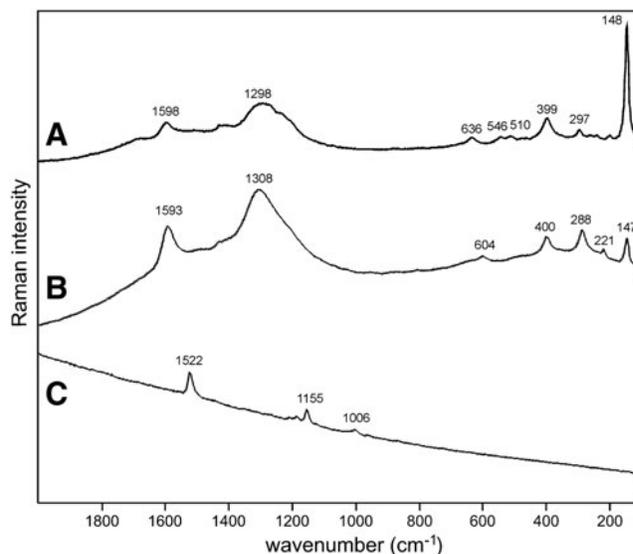
**FIG. 7.** Sample 7 (514.5 nm excitation). (A) anatase; (A) and (B) G and D carbonaceous matter bands between 1100 and 1600  $\text{cm}^{-1}$ ; (B) hematite; (C) clear carotenoid signal between 1000 and 1550  $\text{cm}^{-1}$ .
