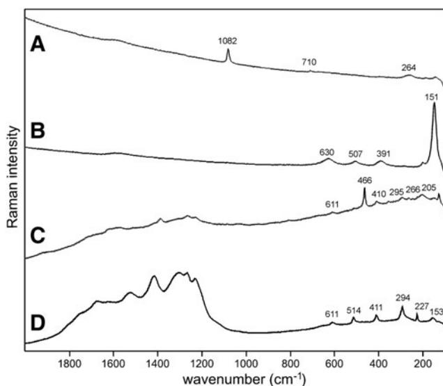
**FIG. 5.** Sample 5 (785 nm excitation). (A) Calcite; (B) anatase; (C) quartz with broad features between 1200 and 1800  $\text{cm}^{-1}$  tentatively suggested as signs of the presence of the highly condensed network of polycyclic aromatic hydrocarbons; (D) hematite (below 700  $\text{cm}^{-1}$ ) with broad features similar to those in the spectrum above.
