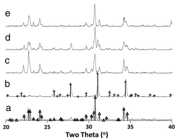
**Fig. 5.** XRD patterns for samples of quenched TCP samples; from bottom to top the samples were: (a) TCP-ACR, (b) TCP-ALF, (c) TCP-MER, (d) TCP-SIG and (e) TCP-WP1. Solid vertical lines topped with triangles and plus signs show Bragg reflections for  $\alpha$ -TCP (ICDD 09-348) and  $\beta$ -TCP (ICDD 09-169), respectively.
