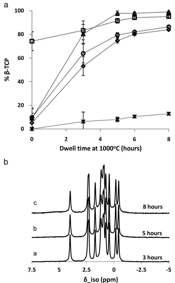
**Fig. 8.** The effect of annealing at 1000 °C on the phase composition of TCP samples. (a) Results, expressed as the percentage of  $\beta$ -TCP formed, elucidated by semi-quantitative analysis of XRD patterns of TCP subject to various lengths of time at 1000 °C: M-ACR (diamonds), M-ALF (squares), M-MER (triangles), M-SIG (circles), M-WP1 (crosses). (b)  $^{31}\text{P}$  MAS NMR spectra of TCP-WP1 annealed at 1000 °C for 3, 5 and 8 hours.
