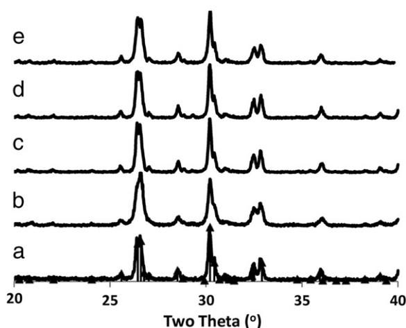
**Fig. 1.** X-ray diffraction patterns for samples of monetite ( $\text{CaHPO}_4$ ) used in this study; from bottom to top, the samples were: (a) M-ACR, (b) M-ALF, (c) M-MER, (d) M-SIG and (e) M-WP1. Bragg reflections shown correspond to monetite as detailed in ICDD card number 09-080.
