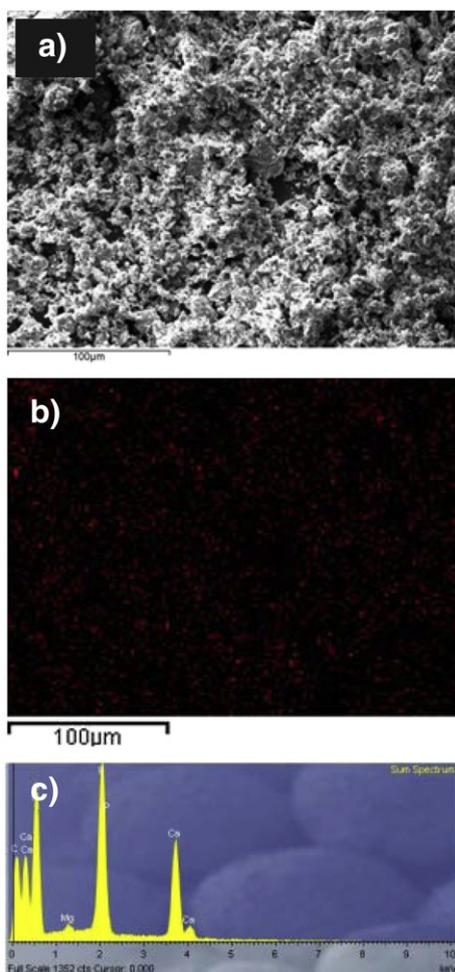
**Fig. 4.** Elemental analysis of a representative monetite sample; (a) low-magnification SEM image of the sample M-MER (from Merck), (b) magnesium signal (red) from EDX mapping of sample image shown in Fig. 4a, (c) EDX spectrum collected on image shown in Fig. 4a.
