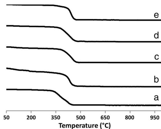
**Fig. 2.** Normalised thermogravimetric curves showing mass loss events for all samples; from bottom to top, the samples were: (a) M-ACR, (b) M-ALF, (c) M-MER, (d) M-SIG and (e) M-WP1.
