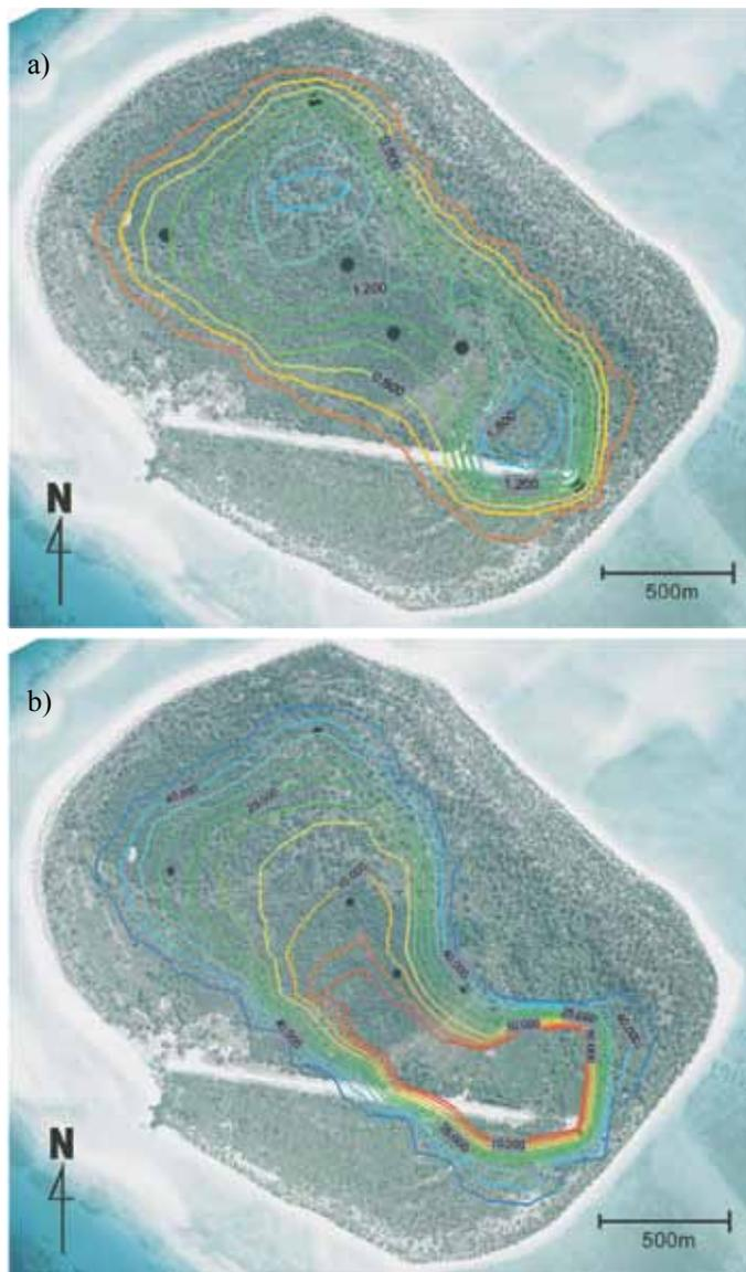
Figure 3. Piezometric (a) and electrical conductivity (b) contour maps of Grande Glorieuse groundwater. The former are presented as lines of equal potentiometric level (in meters above MSL), the latter as lines of equal electrical conductivity (in  $\mu\text{S}/\text{cm}$ ).
