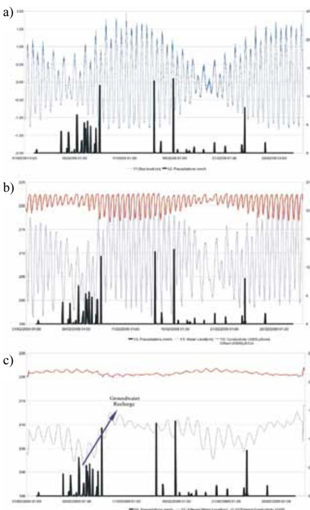
Figure 4. Sea level, rainfall, groundwater level and conductivity at borehole GW2 on Grande Glorieuse island.
