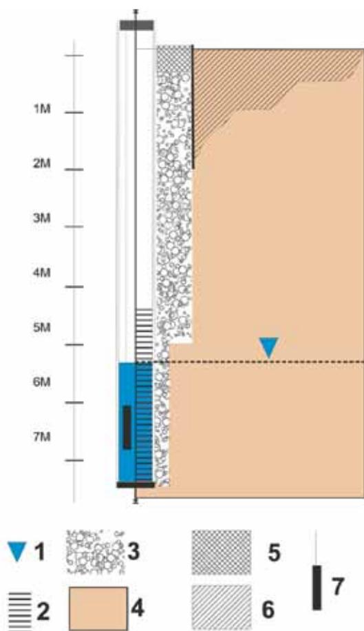
Figure 2. Typical borehole design employed on Grande Glorieuse. 1, water level; 2, well screen; 3, sand pack; 4, terrain; 5, cement grout; 6, backfill with clay ; 7, CTD Diver (datalogger).
