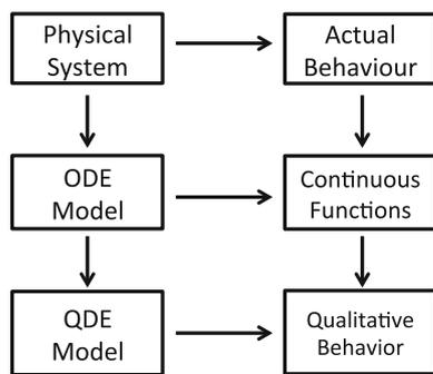
**Fig. 3** This diagram is obtained from Kuipers (1993). The diagram shows that all models are abstractions of the world. Qualitative models are related to ordinary differential equations, but are more expressive of incomplete knowledge
