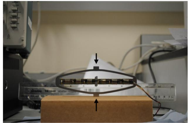
**Fig. 2** Photograph of the composite, high-displacement APA500L piezoelectric actuator used in this work (as sourced from CEDRAT Technologies), showing its relative scale/size against a ruler
