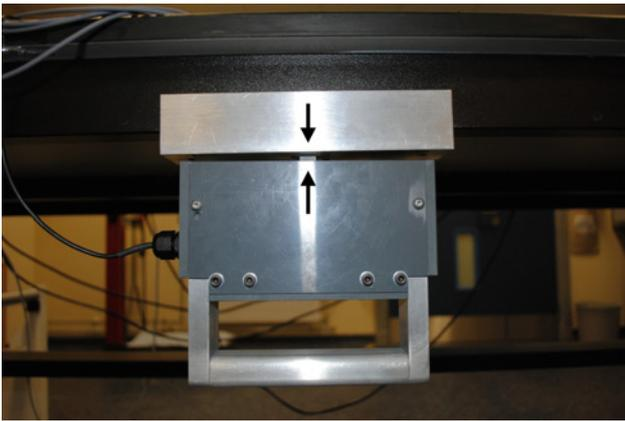
**Fig. 1** Photograph of the ULV device attached to a side of the table from underneath. The arrows explain the location of the piezoelectric actuator inside the casing; the top and bottom arrow signs on the piezoelectric actuator (Fig. 2) correspond to the upper and lower arrow signs on the casing
