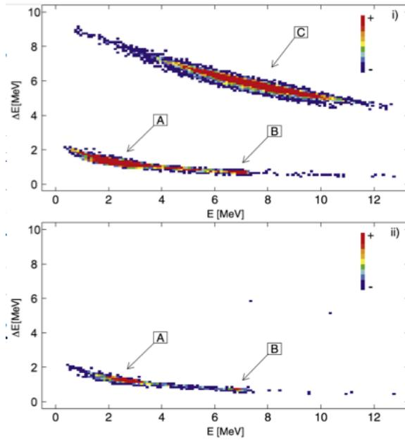
**Figure 2:** Plot of the energy signals recorded in the thin (transmission) and thick (stopping) components of the detector telescope. The labelled groups represent the elastic protons emitted from the back of the front window and the front of the back window (A), the elastic protons emitted from the front of the front window (B), and the elastically scattered  $\alpha$ -particles (C). Upper panel gas in; lower panel gas out.
