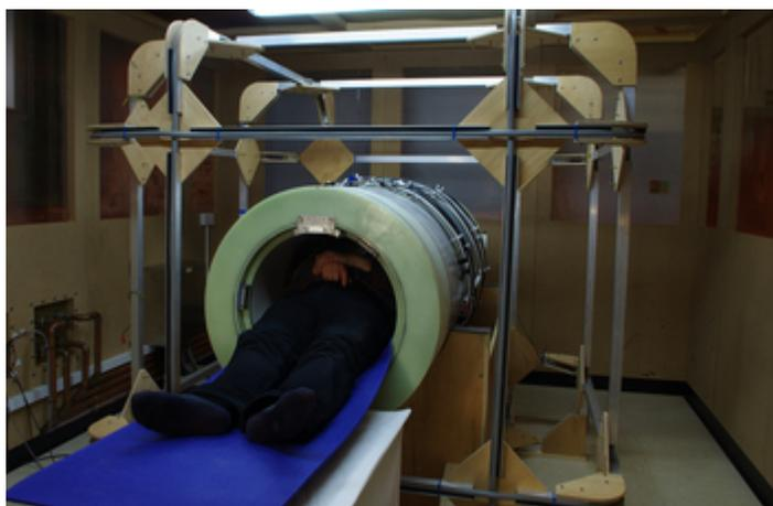
Fig. 1: our magnet consists of three copper coils, co-wound on a cylindrical former, and potted in epoxy resin (Tesla Engineering Ltd, Storrington, UK). At 2040 mm long, 500 mm bore, it is suitable for human subjects. The magnet has a bare inductance of 5 mH and resistance of 85 m $\Omega$  per channel, each requiring 650 A to attain the 0.2 T field specified. The current is supplied by a purpose-built bank of high-power gradient amplifiers (International Electric Co. Oy, Helsinki, Finland).
