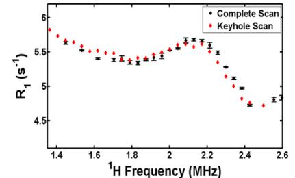
Figure 1: Dispersion curves for a phantom of cross-linked BSA obtained using the keyhole method (red diamonds) show good agreement with results obtained using a conventional field-cycling spin-echo sequence (black circles).
