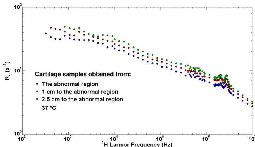
**Figure 1.**  $R_1$ -dispersion curves of 3 samples of cartilage obtained from the knee of a patient suffering from osteoarthritis, from the abnormal region (blue dots), and distances of 1 cm (green dots) and 2.5 cm (red dots) to the abnormal region respectively. The calibration extends the range of minimum measurement frequencies down to 400 Hz (corresponding to a magnetic field of *ca.* 9.4  $\mu\text{T}$ ).
