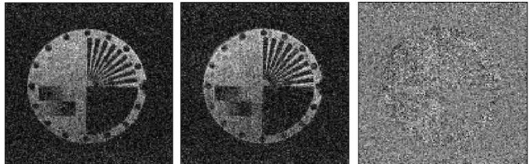
Figure 1: Left: a conventional field-cycling gradient echo 128x128 phantom image acquired using an evolution field of 40 mT. Middle: keyhole image of the same phantom acquired at the same evolution field. Right: The difference of the two images.
