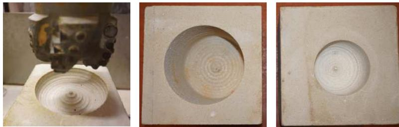
Fig. 6. Examples of rock samples showing the patterns caused by the dynamic interactions with a drill-bit. The left panel shown one of the drill-bits used in our studies having 5 blades with their uneven distribution. As can be seen there is no vertical periodic patterns on the circles forming bottom hole.
